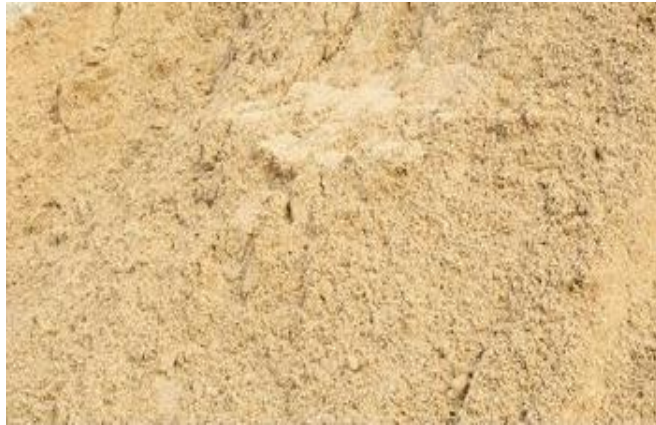
Figure 1: Hill Sand used as Fine Aggregate in this Study
