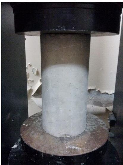
Figure 4: Compressive Strength Test Setup
