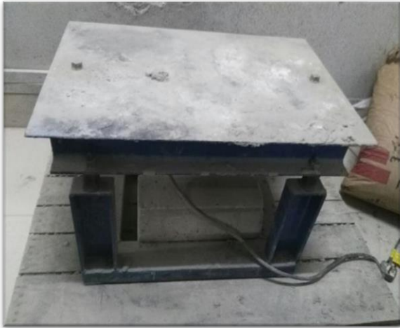
Figure 3: Vibrating table used for compaction of concrete
